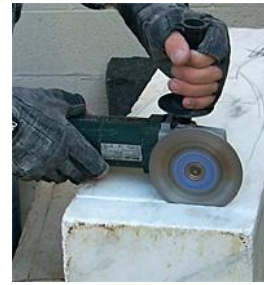
Making cuts with an angle grinder
